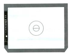
After selecting the aperture, and depress the Shutter Release Button halfway, LED's will illuminates in the viewfinder, indicating both the metering mode ("AV or "SP") and the appropriate shutter speed for the preselected aperture.
