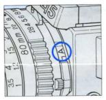
3. Before metering, check that the lens A.M. lever is set at "A". When it is set at "M", proper AE exposure cannot be obtained.
