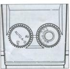
4. Set the Metering Mode Selector to "AV" for Averaged metering, "SP" for Spot metering, or "AUTO A-S" for AV-SP Auto-Shift metering.
